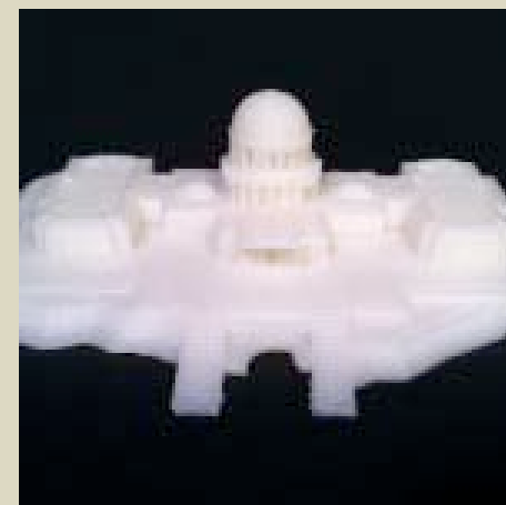
Photo: 3D model US capital, image downloaded from Google Earth, converted in Sketchup and printed using made Solidoodle 3D printer. Solidoodle.com .
